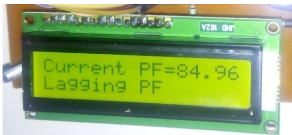
Figure 9 Lagging PF detected by system
