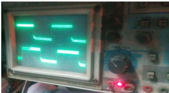
Figure 8: V and I waveforms when load is inductive
