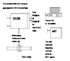
ScanData manufactures an Automatic Reporting Terminal, the ART, which connects to a dialing telephone line and automatically receives reports from any SMR and M-system RTU. The ART automatically answers incoming calls. performs the necessary hand shakes and then sends the incoming report to a printer connected to the ART.
