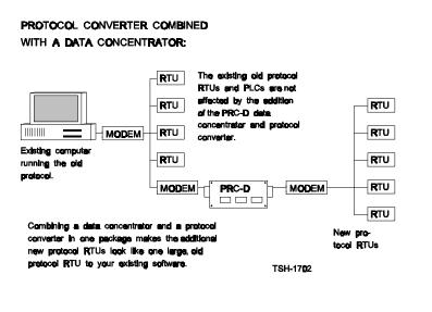
The advantage of this approach is that virtually any number of new RTUS (all communicating in a modern protocol) can be made to look like one or existing more protocol large RTUs to your system.
