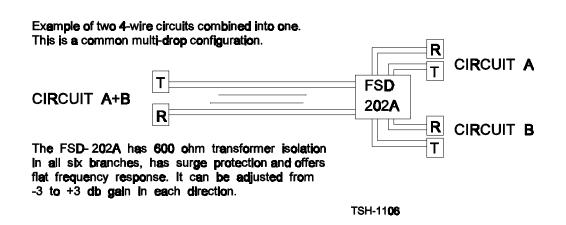
The ScanData FSD-202-A splitter and combiner (multidrop) amplifier is designed for this type of service. It is connected to the modem line input and output terminals. It works on both radio and cable circuits. It splits the modem's line output 2-wire into two 2-wire circuits, one to the cable or radio as before and one to the RTU. It also combines the two incoming 2-wire circuits, one from the RTU and one from the cable or radio into one 2-wire for the modem's line input.
