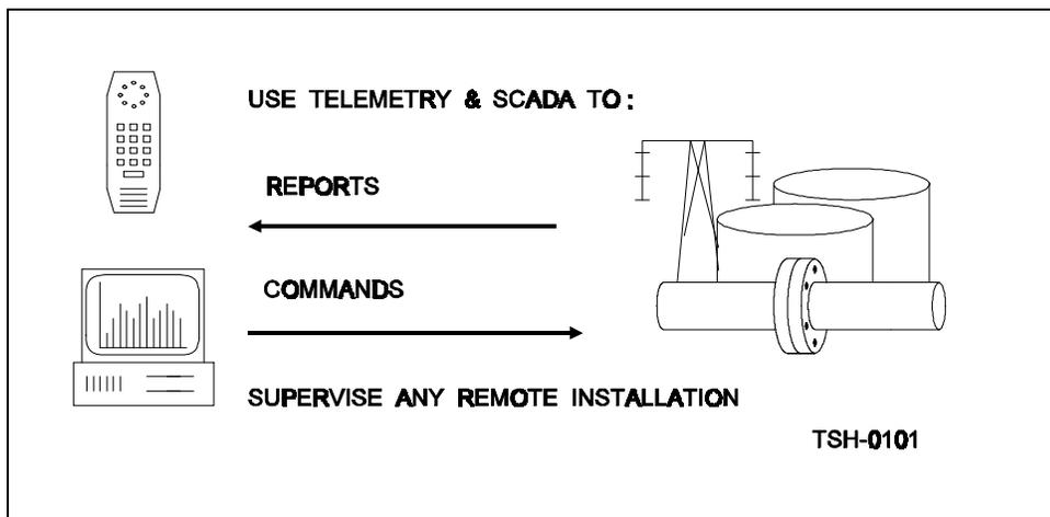
To take a modern example: Say you have a water tank on a hill and a pump at a water well below the hill. Without telemetry, you will have to send your man Charlie out to the tank. He measures the level and comes back and reports. If the tank is not full, you send Charlie out to the pump with instructions to run it for as long as you think it will take to fill the tank.
