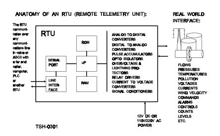
The RTU also converts incoming signals from another RTU or from a central computer into real world output signals to turn relays on and off, start and stop motors, position valves, etc.
