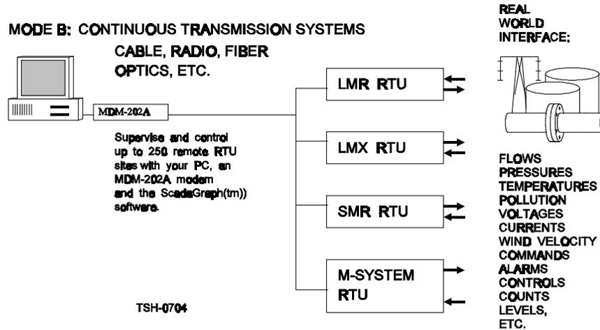
The pressures, temperatures and flows in these pipe lines have to be monitored continuously, generally over computer graphic screens or over large mimic panels that are manned continuously.
