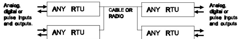
In back-to-back or signal multiplexer mode, two or more RTUs send and receive analog and digital signals from point to point.
