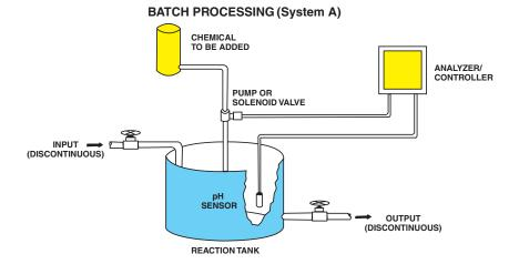
The final control element can be a pump or an ON/OFF valve. Sizing of the final control element is complicated and depends on many factors. This is one situation where a titration curve can be invaluable. In many cases, it may be necessary to use two final control elements, each delivering different amounts of chemical and having different setpoints. For example, one valve may deliver 1 GPM of caustic below 3 pH and another may deliver 0.1 GPM of caustic below 4 pH.
