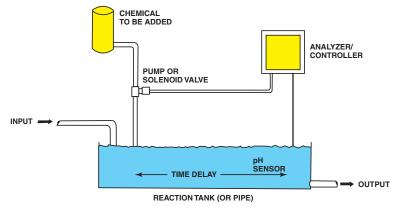
The cycle time should usually be less than the delay time of the system so that a series of shots are in the tank and gradually mixing. By the time chemical reaches the sensor, it should be mixed enough so that the sensor does not measure large variations in pH.
